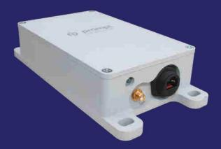
The Prompt Receiver Unit is a machine that collects various data from the activity monitoring tag and delivers it to the server for processing. It is also used for setting various parameters of the activity monitoring tag which has been uploaded from the server. It will also be used to upgrade the sensor's firmware and keep all information updated.
